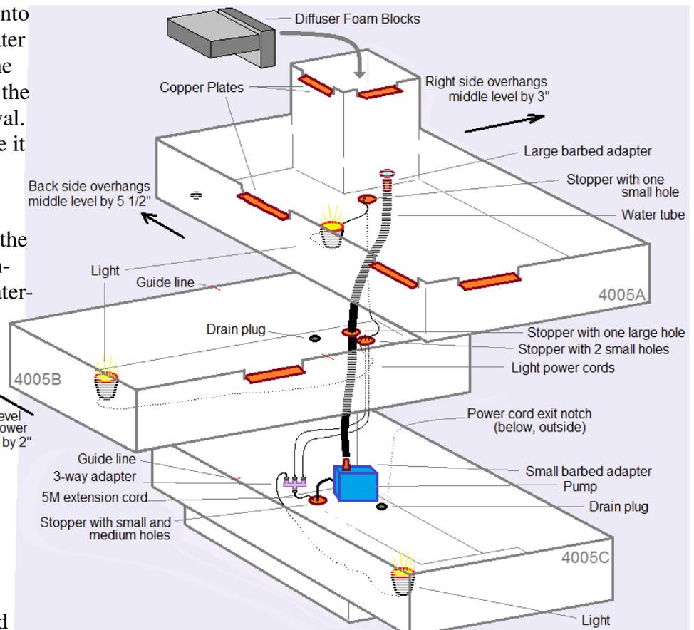
tops of both the back and front wall of the 4005B which will help you line up the 4005A. It should be just a little more than halfway over the 4005C basin.
