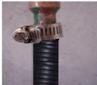
5) Prepare to attach spray bar by holding clamp at top of tube coming up out of Grotto .....
