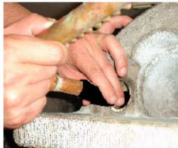
then inserting feed pipe of spray bar into tube .....
