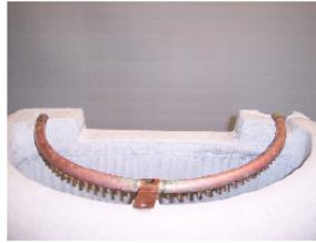
10. Lay the copper spray ring across the top of the wall unit as shown.
