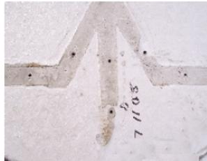
13. Underneath the 4226A Top you will see this pattern with six screw holes. Screw in the six light brackets here.
