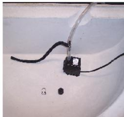
4. Push short clear tube onto pump adapter. Push straight end of tee into other end of short clear tube. Then push longer clear tube onto opposite end of tee. Push black tube onto middle leg of tee. Secure this connection (and any others) with a clamp.
