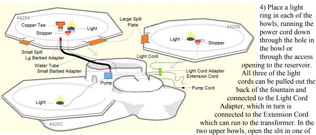
the supplied stoppers, place the power cord (near the light) into the stopper's molded groove, then close and press firmly into the hole. Leave about 1/8" of the stopper visible above the bowl floor for later removal if needed.
