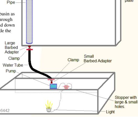
the larger adapter and secure with one of the provided clamps. Lift the top piece over the basin and as others hold it or as it rests on (you must pad this) the basin - push the bottom of the water tube onto the pump adapter and secure with a clamp. Gently set the top piece on the back of the basin.
