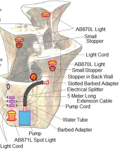
6) Connect the 5-meter-long extension cord to the splitter adapter and run the other end of it out the round hole in the back of the fountain, connecting to the transformer. Make sure a water proof cap is still in place on the remaining sixth junction on the splitter adapter.
