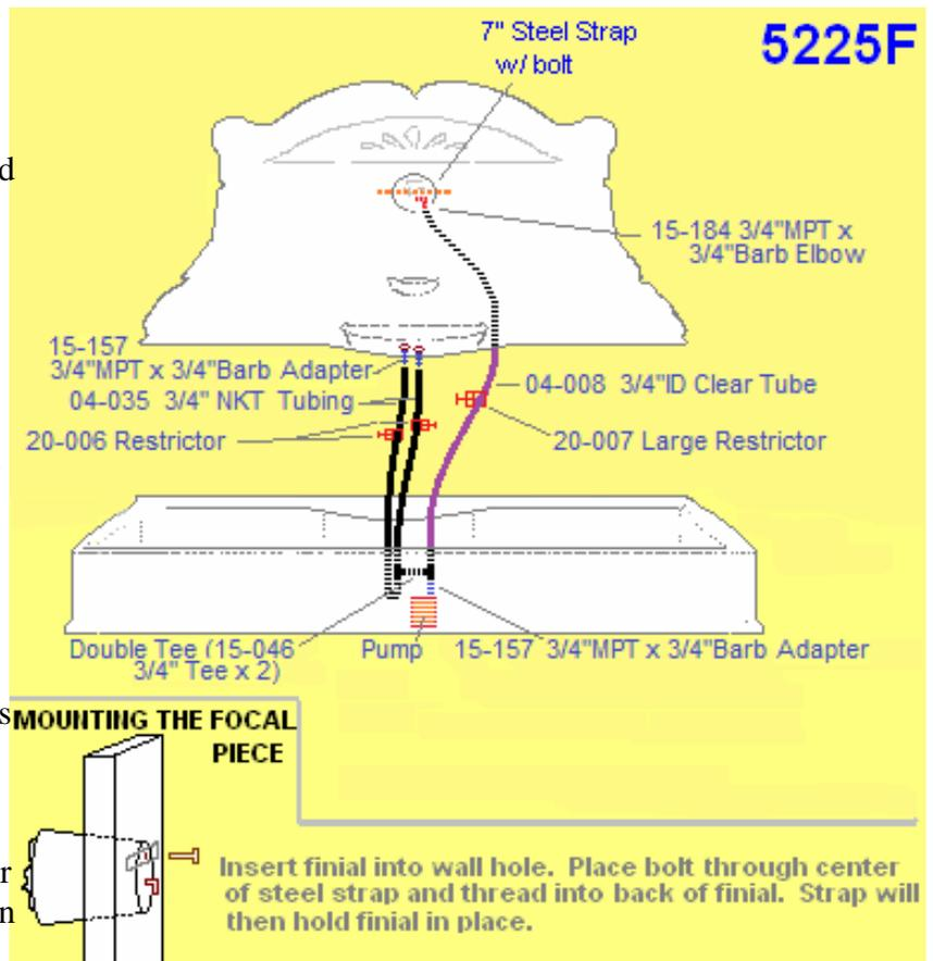
6) Attach the three flow restrictors to the other three tubes, tightening just enough to hold them in place. (The larger restrictor should be placed on the clear tube.) Then drape the clear tube over the back of the basin just as you did with the power cord.
