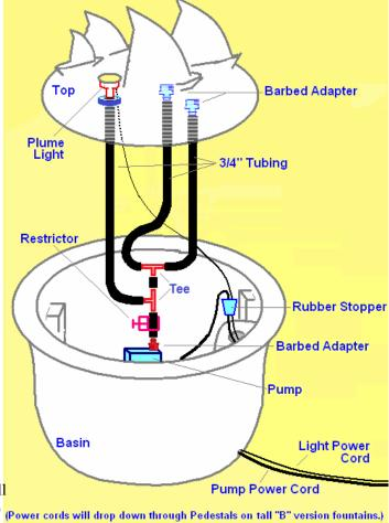
the two remaining long tubes onto the two end barbs of the second tee.
