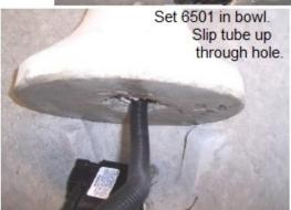
Hold tubing exiting above the 6501 with a stopper. Press in firmly. Attach larger adapter to the end of the tube, barb side into tube.
