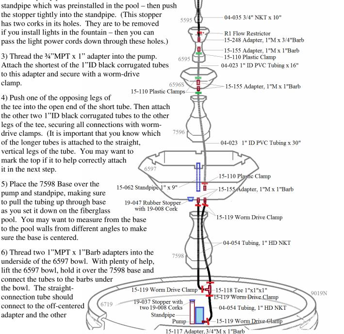
tube should connect to the adapter in the center. Connections should then be secured using the worm-drive clamps. Set and level the bowl with shims if necessary.
