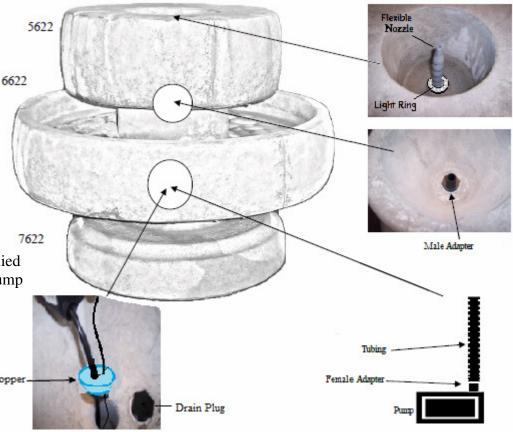
Fill the bowl with water. Read your pump instructions. Plug in the pump to see the fountain work. If the pump does not immediately push water there may be an "air lock". Such an air lock can be removed easily by unplugging and re-plugging the pump a few times. 4/19
