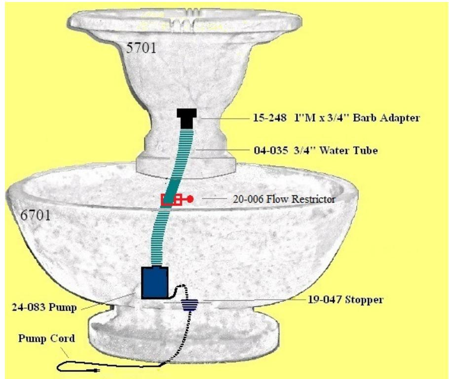
5) Thread the 15-248 1" male x 3/4" barb adapter into the underside of the 5701 top unit.
