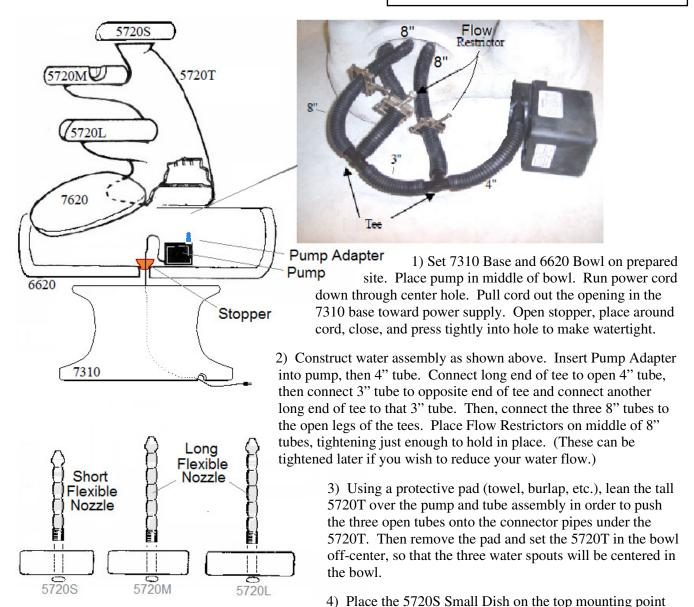
of the 5720T. Thread the Short Flexible Nozzle down through the hole into the coupling in the 5720T. Repeat this process for the 5720M Medium Dish and the 5720L Large Dish, using the Long Flexible Nozzles. Turn the top small dish to pour into the medium dish, which will pour into the large dish. Finally, hide your pump and water assembly by placing the 7620 Pump Cover over it.
