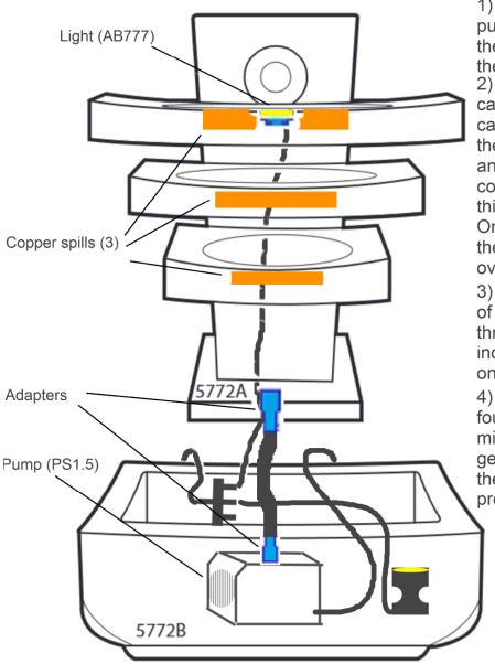
1) Place the pump in the basin, drape the pump cable out the back of the basin. Affix the smaller of the two included adapters to the top of the pump.
