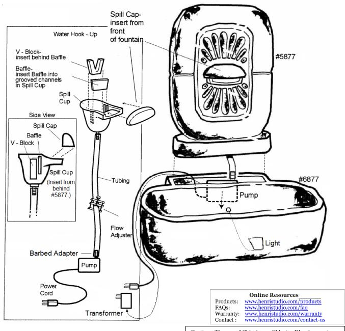
Once all is in place, fill basin with water. Read pump and light instructions. Turn on the pump and light. If it does not immediately begin working, there may be an "airlock" within the impeller chamber. Simply unplug and plug in a few times and it should start.
